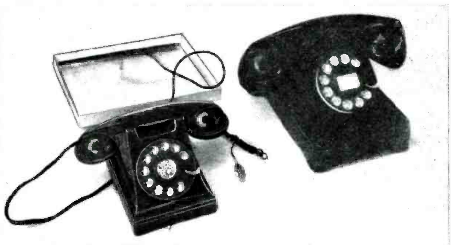
Fig. 3—Toy radio at left is tuned by turning the "telephone" dial. Standard phone at right.
