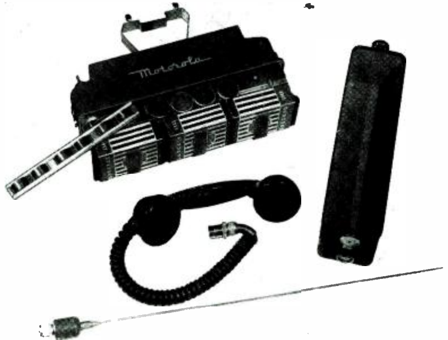
This is the portable radio set. The antenna, handset and bottom cover have been removed.
