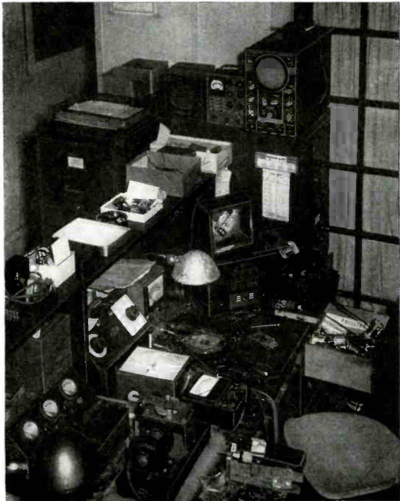
Intercoms, hearing aids, and amplifiers are tested and repaired on Audiphone's bench.
