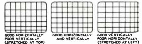
Fig. 3—Grid pattern is good linearity check.
