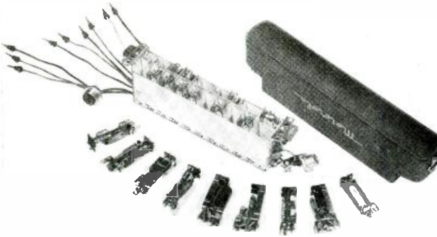
The top cover and nine of the plug-in units have been removed to show chassis construction.
